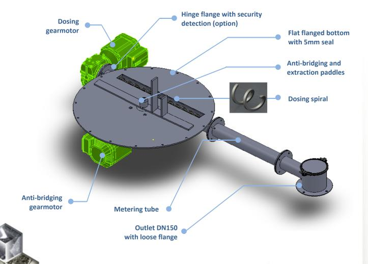
This unit works easily connected beneath standard hoppers capacity 150 / 300 / 500 liters or with special connection beneath silos, mixers, bulk bags discharging station
